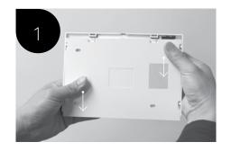
Slide the mounting plate off the console.
