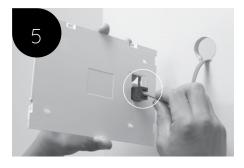
Pull in the cable from the hole and connect it to the RJ12 socket.
