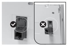
Ensure the RJ12 is properly aligned when connecting it to the console.
